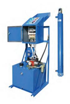
Actuator 90-0300 is applied oscillating motion with fixed amplitude according to the cylinder stroke. Movement of the cylinder rod can be continual or with a pause at the end position. Changing direction of the movement carried out without proximity switches so the device is insensitive of the dust and humidity.
