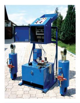
Actuator 90-0250 is applied for automatic correction of lateral deflection of the conveyors. The hydraulic cylinders swivel the band roller according to the signal from proximity detectors and keep the band in proper position. Control valve block assembled directly on the cylinder prevents the creep movements.
